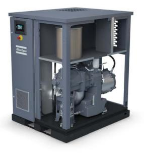
The variable-speed drive ZS 4 VSD<sup>+</sup> screw blowers compress the air with its efficient permanent magnet motor (located in the back of the machine, half right in the picture) by around 10% more efficiently than the previous generation. And they need less floor space. (Photo: Atlas Copco)
